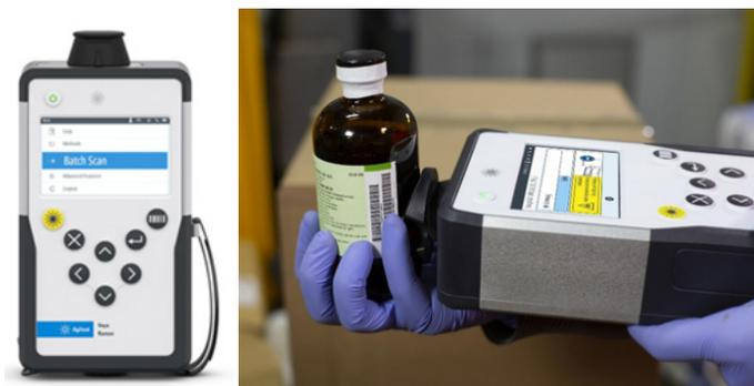
**Figure 1.** The Agilent Vaya Raman handheld spectrometer with SORS technology being used to identify materials/solvents through an amber bottle.
